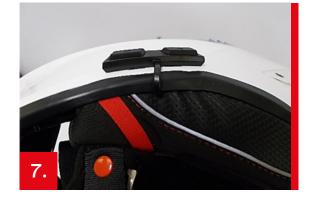
During the comfort cheekpads assembling, pass the flat cable of the remote control between the cheekpad pp plate and the shell. The remote control must remain accessible outside the helmet.
