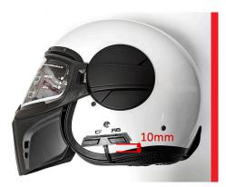
Fit the keypad on the left side (helmet on), approximately 10 mm from the lower edge of the shell using the provided adhesive. Make sure that there is full contact surface between the adhesive keypad and the outer shell.
