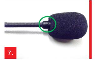
Adjust the microphone's position by deforming its boom.
