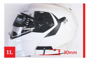
Fit the keypad on the left side (helmet on), approximately 30 mm from the lower edge of the shell using the provided adhesive. Make sure that there is no interference with the chin guard and full contact surface between the adhesive keypad and the outer shell.
