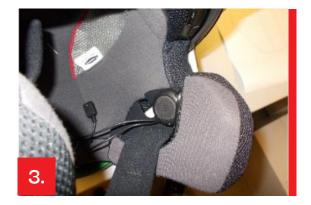
Repeat the operations performed for the right (R) speaker for positioning the left (L).
