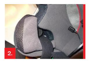
Place the right speaker (R) on the cheekpad's pp plate after applying the adhesive round shaped velcro included in the package.
