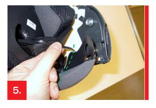
Pass the flat cable of the remote control cable between the neckroll's pp plate and the shell. The remote control must remain accessible outside the helmet.
