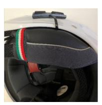
During the comfort cheekpads assembling, pass the flat cable of the remote control between the cheekpads's pp plate and the shell.
