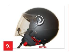
Fit the keypad on the left side (helmet on), approximately 10 mm from the lower edge of the shell using the provided adhesive. Make sure that there is no interference with the chin guard and full contact surface between the adhesive keypad and the outer shell.
