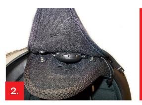
Place the right speaker (R) behind the cheek pad at the holes using the velcro on the back of the speaker.
