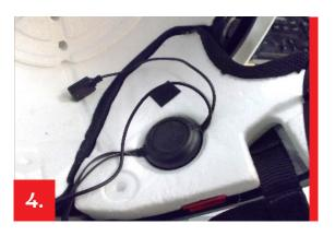
Repeat the operations performed for the right (R) speaker for positioning the left (L). Warning the left speaker must be rotated of 180 ° before being placed in the seat.
