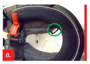
Place the USB socket between the removable cheek pads and the neckroll.
