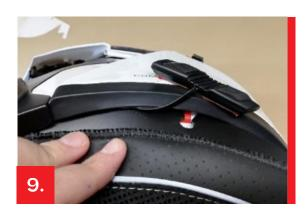
Pass the flat cable of the remote control between the neckroll's pp plate and the shell. The remote control must remain accessible outside the helmet.
