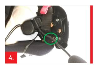
Position the microphone by passing the boom under the chinstrap that will be housed in its seat.
