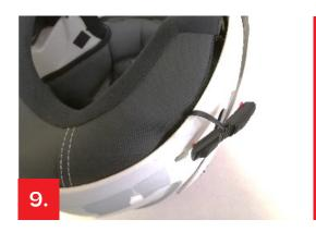
Pass the flat cable of the remote control between the neckroll's pp plate and the shell. The remote control must remain accessible outside the helmet.
