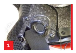
Remove the inner linings as indicated in the helmet user manual.
