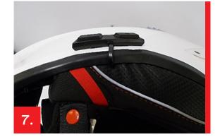
During the comfort cheekpads assembling, pass the flat cable of the remote control between the cheekpads's pp plate and the shell. The remote control must remain accessible outside the helmet.
