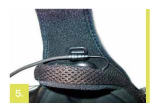
Attach the microphone on the comfort padding with the Velcro on the back of the microphone base.
