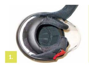
Remove both cheek pads and place the connecting cable between the left and right speaker under the rear cushion.
