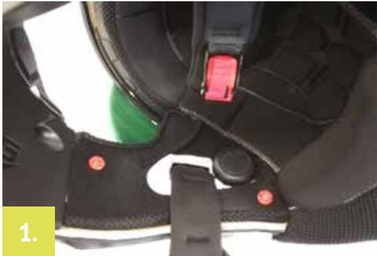
Remove the cheekpads as indicated in the communicator's instruction manual. Place the right speaker (R) in its seat after applying the adhesive round shaped Velcro included in the package.
