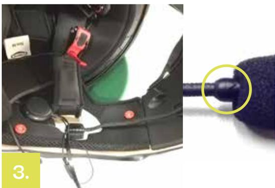
Place the microphone's base in its seat on the left EPS cheekpads.
