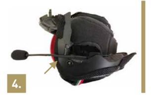
Attach the microphone base to the linings's side plate with the Velcro included in the package. Place the microphone boom over the automatic button.
