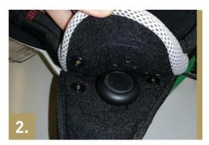
Place the right speaker (R) behind the cheek pad at the holes using the velcro on the back of the speaker.
