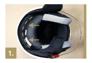
Remove both cheekpads and place the connecting cable between the left and right speaker under the rear cushion.
