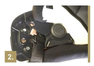
Place the right speaker (R) in its seat after applying the adhesive round shaped Velcro included in the package.
