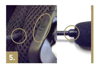
Adjust the position of the microphone by deforming the boom and insert it in the relative seat indicated by the symbol of the microphone on the shell left side.
