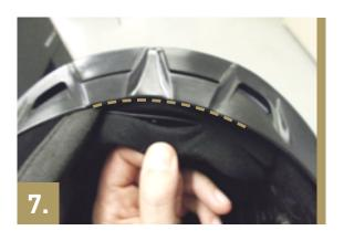
Assemble the inner linings making sure that the microphone, remote control and USB cable are accessible from outside the helmet.
