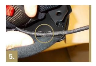
Position the microphone underneath the chinstrap by housing the boom in its seat.
