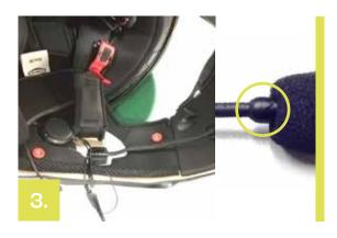
Place the microphone's base in its seat on the left EPS cheekpads.
